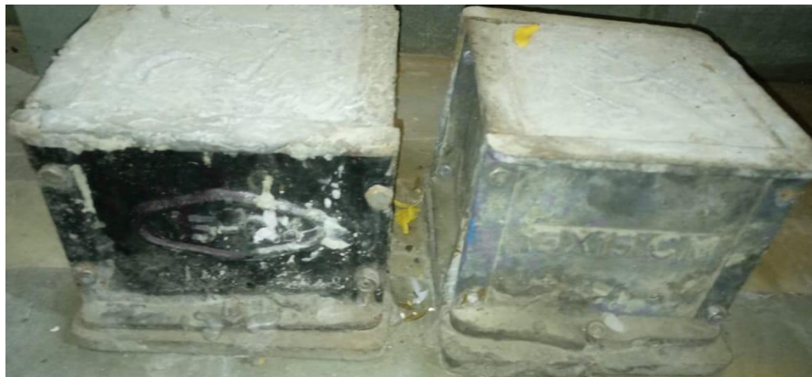
(b) Cubes for strength testing of concrete mixture
