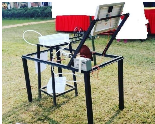
Fig.1: Solar power reciprocating pump
