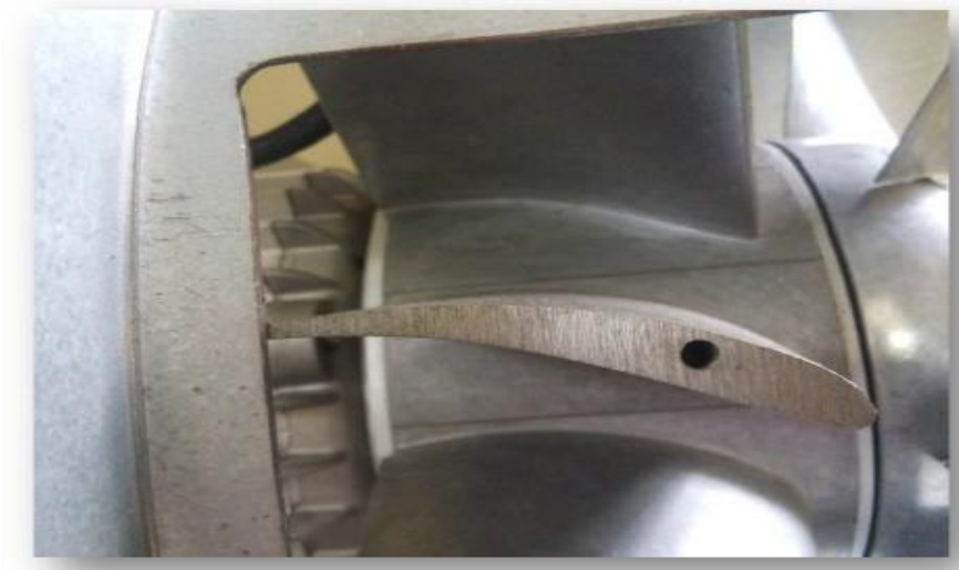
Figure 2.8. Asymmetric Aerofoil guide vanes of actual design
