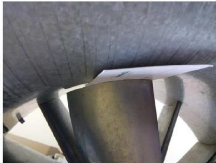
Figure 2.10. Closeup view of blade tip clearance in our design
