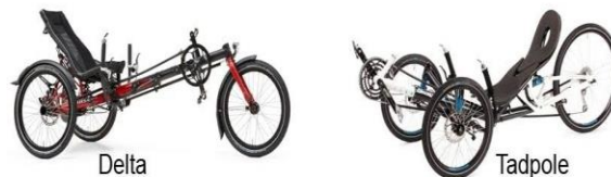
Fig-2 Delta trike & Tadpole trike
