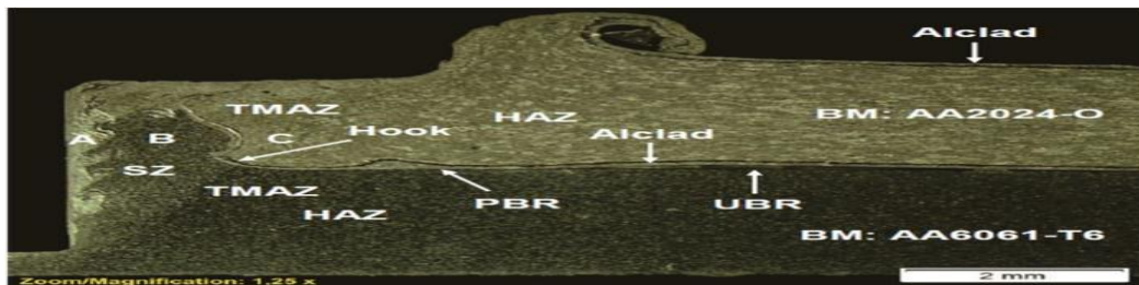
Fig. 6. Cross-sectional appearance of FSS welded dissimilar AA2024-O/AA6061-T6 joint produced using a cylindrical pin at 900 rpm.
