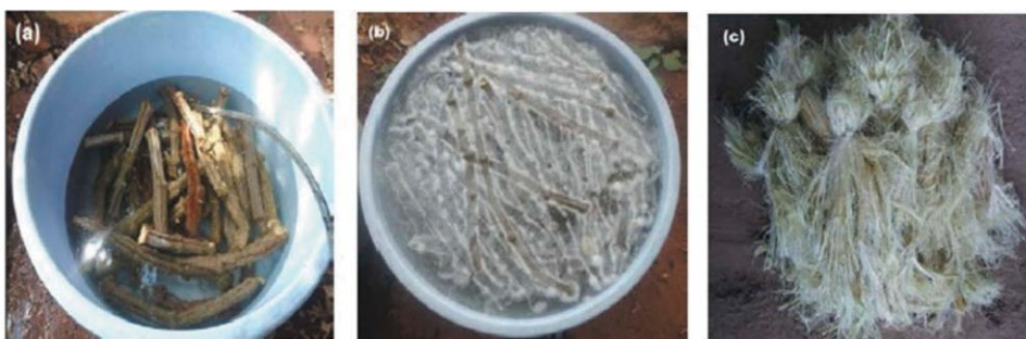
Figure 1. Fiber extraction process (a) sliced CI stems immersed in water (b) CI stems in water after 3 weeks (c) extracted fibers.
