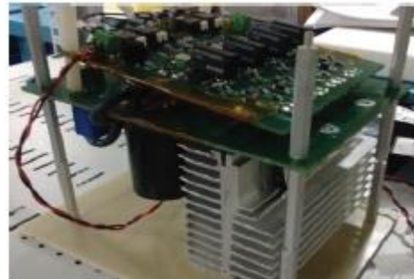
Fig. 8: 1200V/1700V H-bridge Converter Prototype
